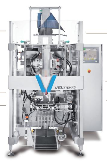
producers with its ability to create 16 variations of doy-style stand up pouches and 55 other bag types, handle bag widths up to 280mm and achieve speeds up to 200 bags/min. The DOS doser is highly recommended for coffee producers.
